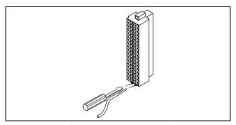
Figure 5. Connecting Wires to the NI 9264 Connector
